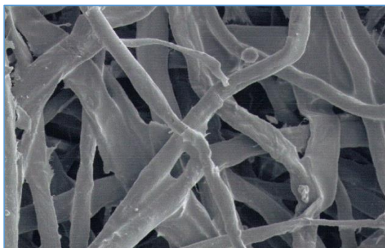
Unused paper element at x270 magnification
